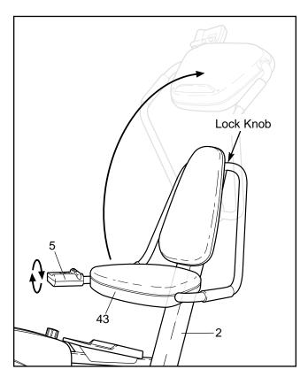
To switch from elliptical crosstrainer to recumbent bike, loosen the Lock Knob (81, not visible). Fold the Seat (43) down and turn the Console (5) so it is visible when you are sitting on the Seat.
